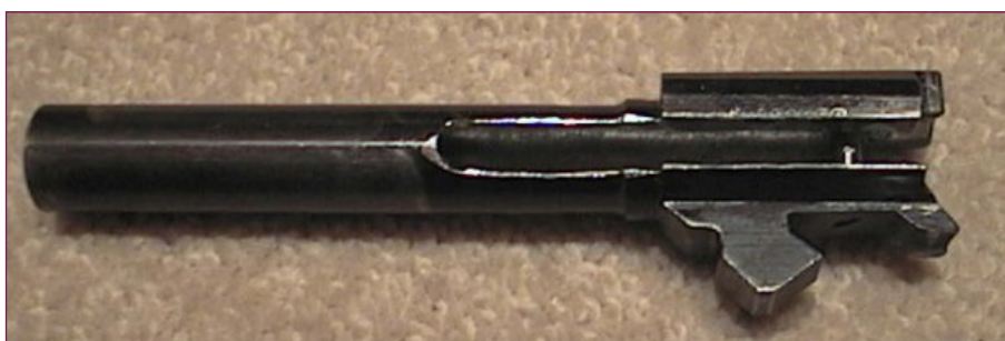
Figure I. A deactivated SIG Sauer P226 barrel demonstrating a slot cut into the feed ramp
