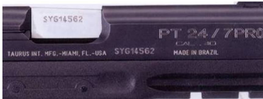
Figure V. Example of an alphanumeric marking on the barrel of a firearm
