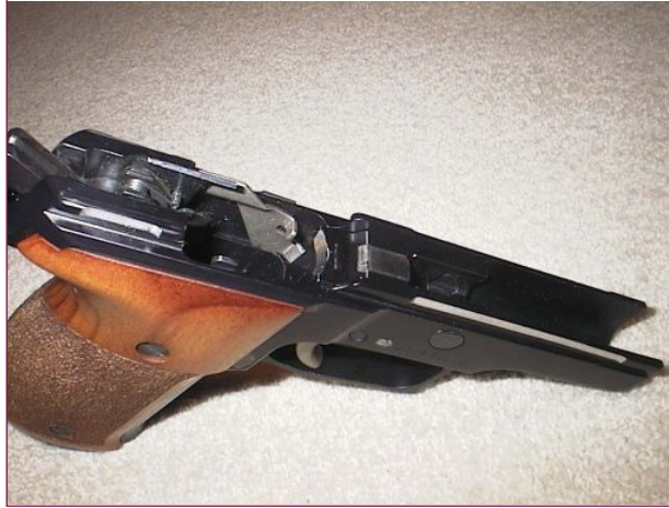
Figure II. A deactivated firearm with two thirds of the frame rails removed and the feed ramp milled out
