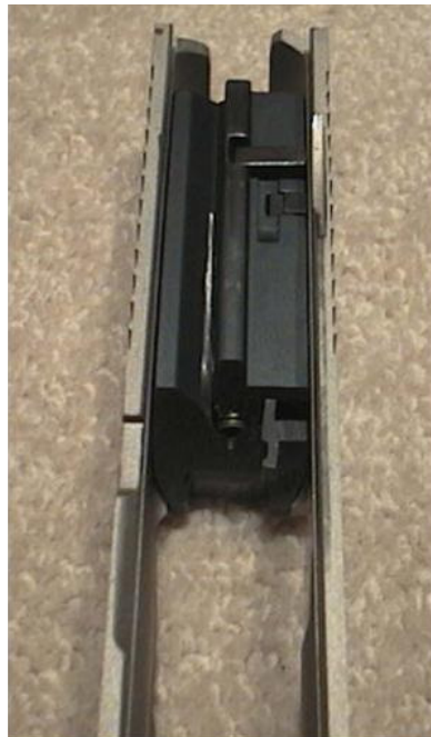
Figure III. Deactivated firearm with the breech face cut off at an angle and the tip of the firing pin removed
