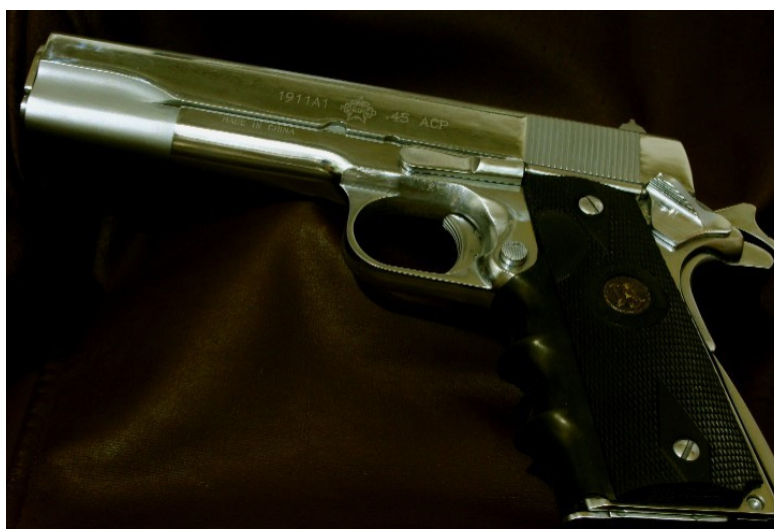
Figure I. Example of a classical marking on the barrel of a firearm
